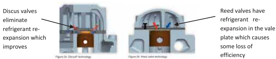
Figure 10: Discus valves vs. Reed valves
