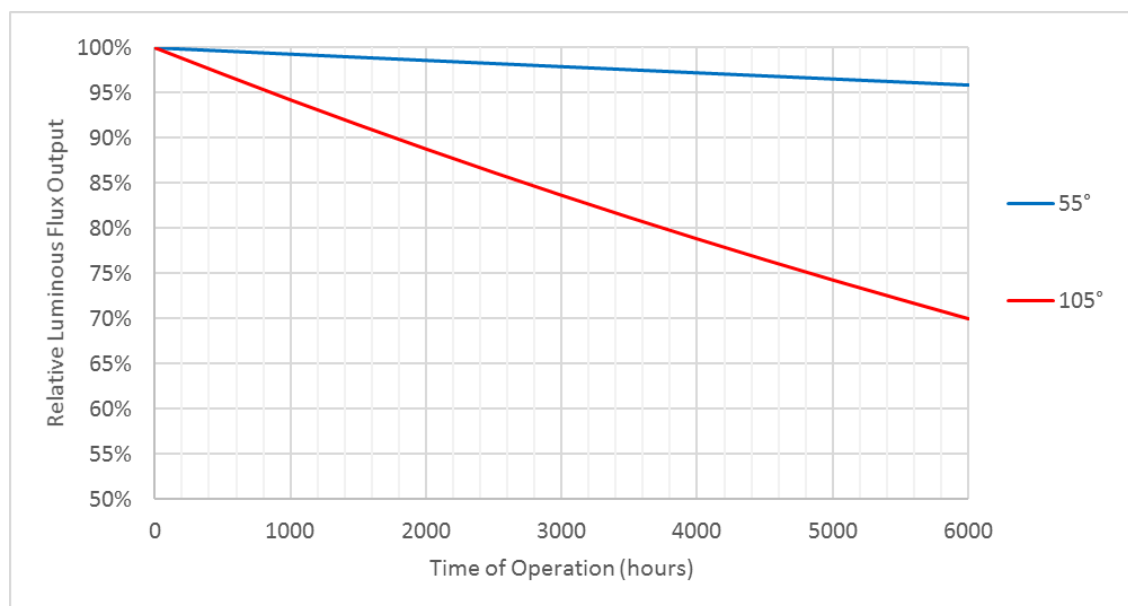
Figure 10: Measured LED lumen depreciation rates for LED module at different operating temperatures but same drive current
