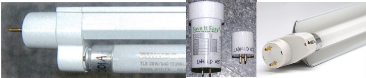
Figure 20. Examples of T8 to T5 adapters. These are inserted into a T8 luminaire in place of a bare T8 lamp. [Left] shows bare batten style adapter; [centre] shows end cap style such that T5 is inserted bare; [right] shows batten style with inbuilt reflector.
