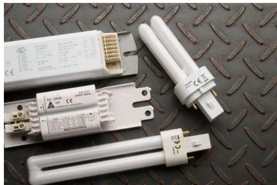
Figure 3. Non-integrated CFLs (right and bottom of picture), electronic fluorescent lamp ballast (left top) and a magnetic fluorescent lamp ballast (left centre).
