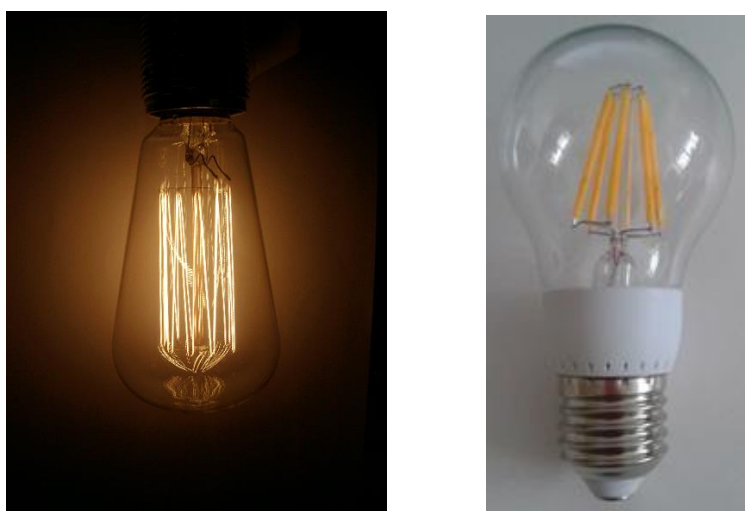
Figure 24 – Old style tungsten / carbon filament (left) alongside LED equivalent (right)
