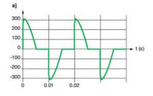
This type of Leading Edge dimmer was designed to control resistive (analogue) type loads and inductive transformers by "chopping" energy from the leading edge of the sine wave.
