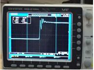
With enough "ring-up" the transformer may exceed the maximum voltage rating of any components causing lamp flicker or component failure.
