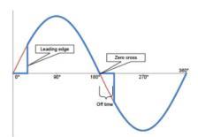
Correct reference of the zero cross over triggers or "clocks" the introduction of the energy reduction in the leading part of the half cycle.
